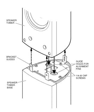
STEP 7 — Turn stand over and slowly lower the tower assembly onto the stand, being careful to insert the alignment pins into their receptacle guide holes.
