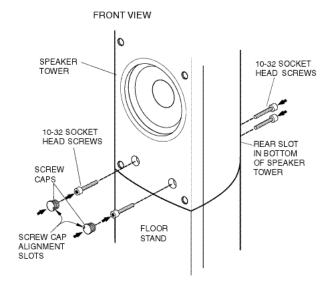
STEP 8 — Fasten the four 10-32 Socket Head Screws through the tower base as shown; two through the front baffle and two in the rear slot. Press flush into place two screw caps to hide holes in front-baffle base. Make sure that the alignment slots point toward the center to ensure that the surface curve matches that of the baffle.
