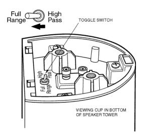
STEP 1 — When using the tower as a surround speaker, set Toggle Switch in tower cup to "Full Range." When using as a front channel,set Toggle Switch in tower cup in bottom to the "Full Range" position. Please consult the Prelude MTS Subwoofer manual for exceptions to this setting.
