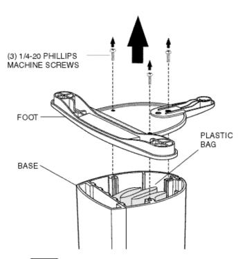
(STEP 4) – To add greater stability to the tower stand, add sand (not included) in the plastic bag provided in the tower base. Turn the base upside-down and remove the (3) 1/4-20 Phillips screws holding the foot onto the base.
