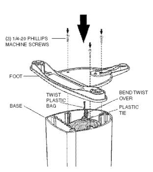
STEP 6 — Seal the plastic bag, making sure to tuck it back inside the base and place the previously removed foam pad on top of the sealed bag. Replace the foot with the same 1/4-20 Phillips screws.
