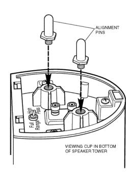
STEP 2 — Screw alignment pins into cup in bottom of tower. Use two per tower. Screw threaded ends into holes and tighten until snug.DO NOT overtighten.
