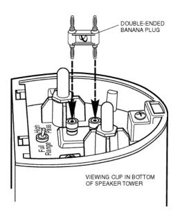
STEP 3 — Insert double-ended Audio Banana Plug into tower as shown.
